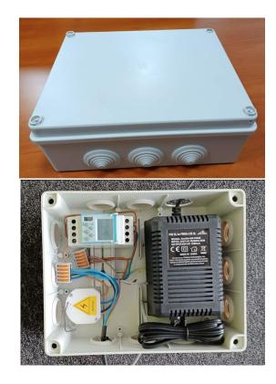
Example of an electrical box equipped and connected with timer, remote control receiver, wago's and power supply – all fit to the box
